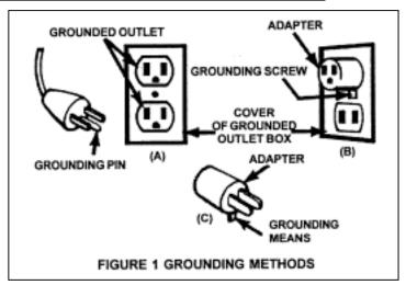
NOTE: The temporary adapter should be used only until a properly grounded outlet can be installed by a qualified electrician.
